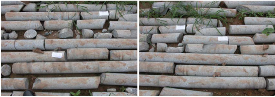
Fig. 3 Cores of the igneous rock
