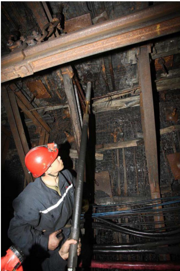
Fig. 4. Photograph of hydraulic fracturing stress test in an underground roadway (Kang et al., 2010).
